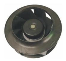
Frame: Aluminum Impeller: plastic (UL 94V-0) Ambient Temperature Range: -10°C ~ +70°C Bearing: Ball Weight: 1500 g
