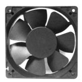
Frame: Thermoplastic PBT UL 94V-0 Impeller: Thermoplastic PBT 94V-0 Ambient Temperature Range: -10°C ~ +70°C Bearing: Ball or Sleeve Termination: Terminals or Lead wire Weight: 172 g
