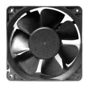
Frame: Thermoplastic PBT UL 94V-0 Impeller: Thermoplastic PBT 94V-0 Ambient Temperature Range: -10°C ~ +70°C Bearing: Ball or Sleeve Termination: Terminals or Lead wire Weight: 301 g
